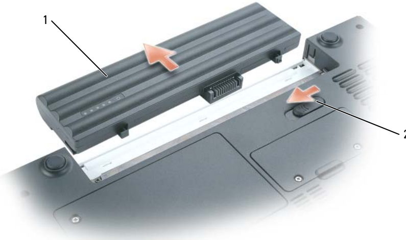
1 battery 2 battery-bay latch release
