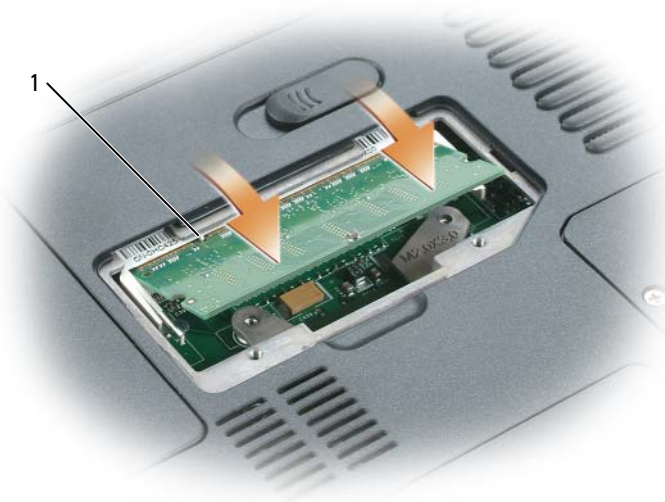
1 tab in connector slot
